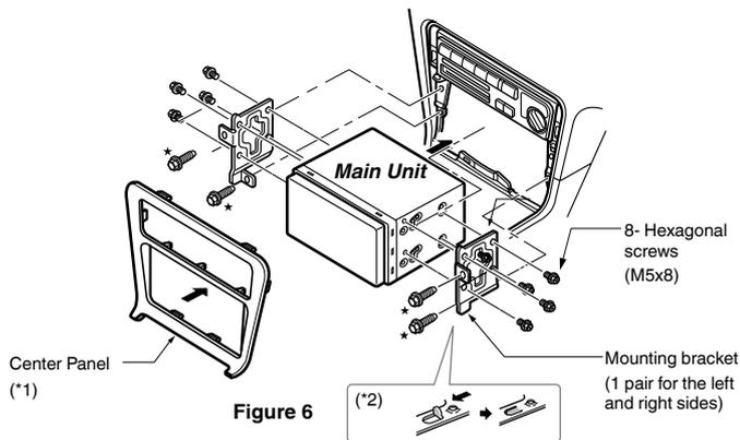
\*1. Some panel openings are too small for the unit depending on the vehicle type and model. In such a case, trim the upper and lower sides of the panel frame by about 0.5 to 1.5 mm so the unit can be inserted smoothly.
