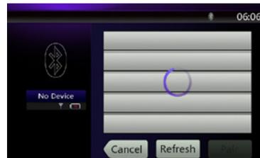
4. Touch your desired Cellular button to select the button for the cellular phone to be registered, and touch [ **22:30** ] button to register for the Bluetooth cellular phone.
