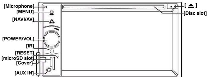
Note: When the [RESET] button is pressed, frequencies of radio stations, titles, etc. stored in memory are cleared.
