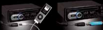
Rear USB enables connection of iPod and USB memory devices. (Only for CZ209A)
